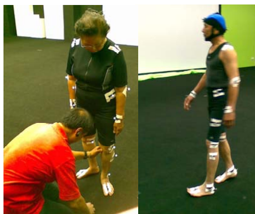
Fig. 2. Marker System (a) a participant was installed with markers (b) the participant was walking during motion data collection.
