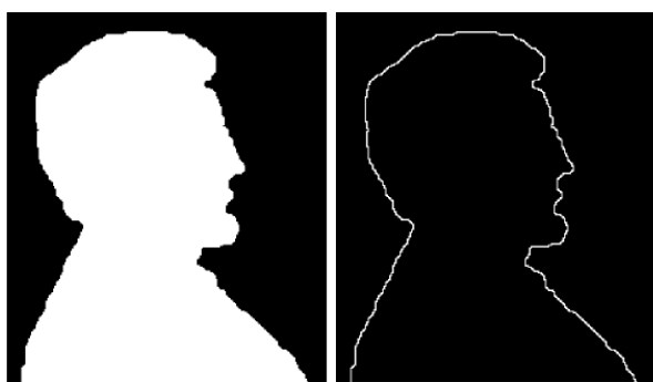
Fig.3 Boundary extraction using 3*3 square element.[4]
