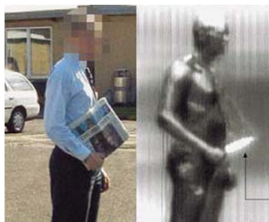
Figure 2.5: terahertz image of men with hidden knife
